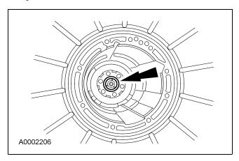
33. Install the No. 6B forward clutch thrust washer onto the forward ring gear hub.
